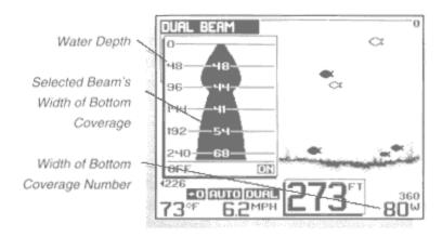
The options in the Transducer menu are "Dual", which uses both transducer elements for transmitting and receiving the sonar signals, "Narrow" which selects ments available in the Transducer menu will be "Left", "Right", and "Both". More information about these options is discussed in "Wide Side Operation".
